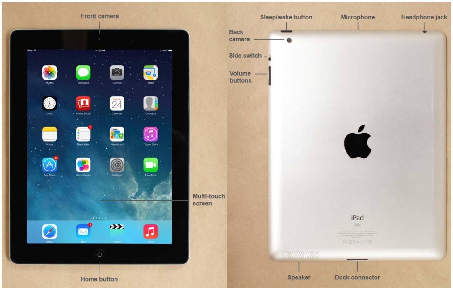
\* If you have the latest version of the iPad, the dock connector will be slightly smaller than the one pictured above. The new connector is known as a Lightning connector, and you'll use a Lightning cable to charge your iPad or connect it to your computer.
